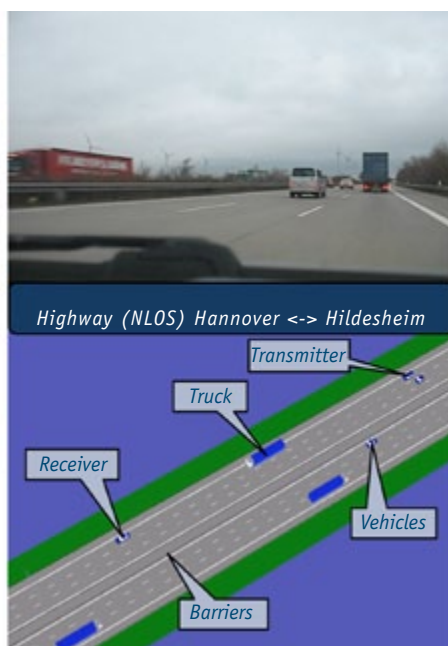
Figure1: Two scenarios with NLOS conditions: highway and inner-city with dense constructions
