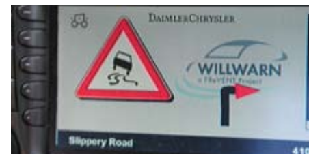
Figure: Example of WILLWARN HMI
